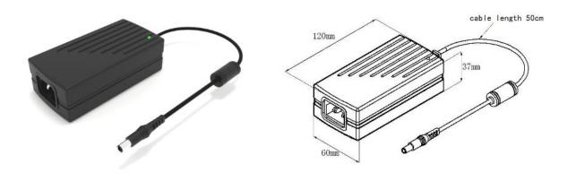
The Universal Diode Laser Module Power Supply with CE-marked provide a well-regulated 5VDC. This autoranging power module can be connected to any 85-264 VAC 47/63 Hz supply. There is an IEC 60320 input socket and a 0.5m output cable terminated with an easy connect/disconnect jack socket. The Headset connector which could also be found in accessories is compatible with the power supply jack.
