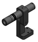
The module mount is used for 19mm diameter diode modules. Loosen the two small set screws on the top half of the module mount to put the laser in. The laser is held firmly by tighten the screws. The module mount base reserved the 4 holes for users to fix the laser on a flat and heat-dissipating surface. Moreover, the module mount can be tilted about 45°.
